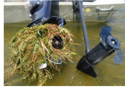
Boat Propeller with Eurasian Watermilfoil
