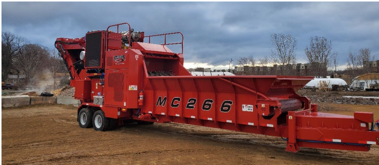
This photo was provided by Papio Valley Nursery, which was awarded funds toward a wood grinder to process 55,000-75,000 yards of wood waste annually. The wood chips will be used for a wood burning broiler system for their greenhouses.
