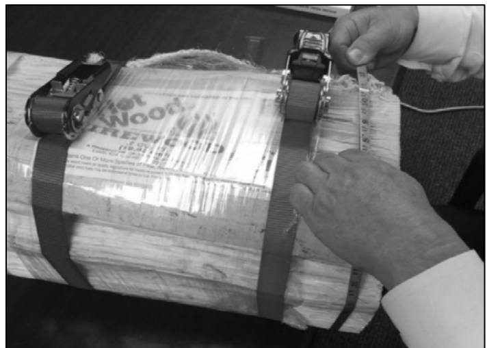
Figure 3-13a. Strapping the Ends of a Bundle.
