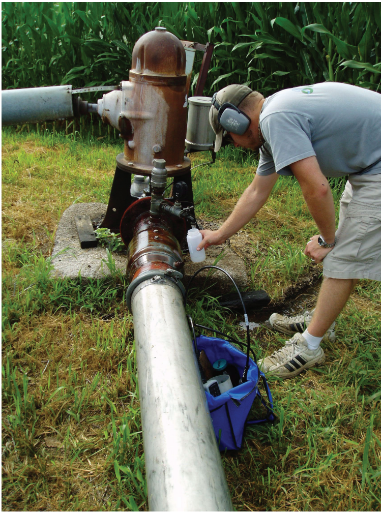
Lower Platte South Natural Resources District sampling an irrigation well.
