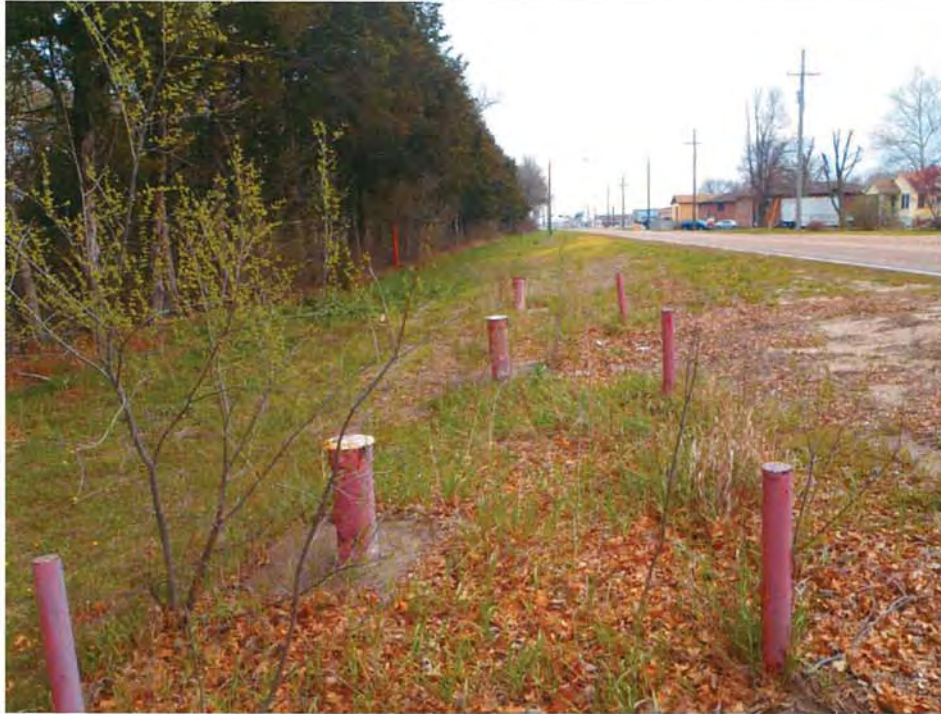
Photo 13: Apparent monitoring wells located along the west side of the assessment property. Looking south.
